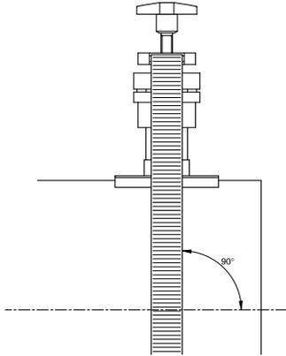
**5.** Make sure that the belt is perpendicular to pipe axis.
