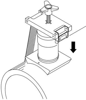
**2.** Insert the positioning tool into the “top load” saddle and place them on the pipe, after completing scraping and cleaning operations (check installation instruction of the fitting).
