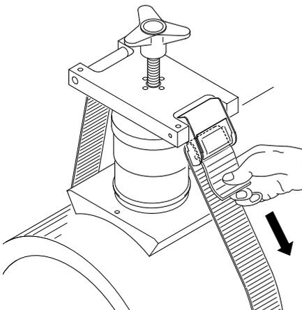
**4.** Insert the belt up in the buttonhole and then pull down to tighten the ‘top load’ saddle on the pipe.
