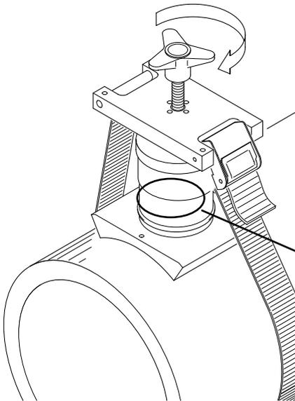
**8.** Remove the positioner by turning counterclockwise the handle and extract the belt from the tightening clamp.
