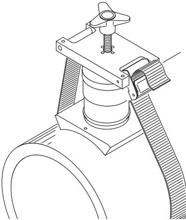
**3.** Pass the belt under the pipe and insert it into the tightening clamp from the bottom to the top, as showed on the figure.
