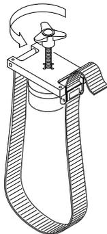
1. Prepare the tool for use by turning counterclockwise the handle until level **A** will reach level **B**.
