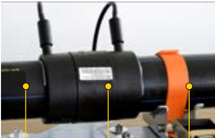
Trac. 1 > Pipe Trac.2 > Fitting Trac.3 > Pipe
