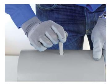
Wait for a cooling time of 1 minute and cut the cap.
