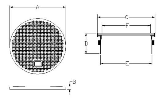
Dimensions for composite manhole cover lids (using legend above)
