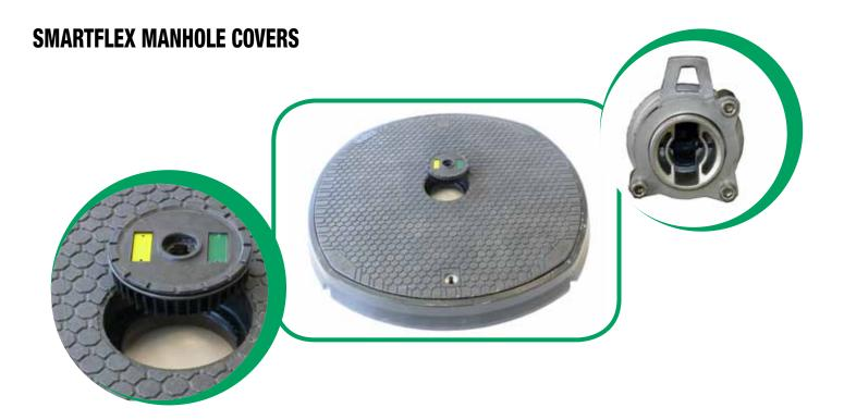
**SMARTFLEX Composite Manhole Covers** are designed to offer a light weight alternative to steel manhole covers. These covers are class C250 (up to 25 tons) and D400 (up to 40 tons) in accordance with EN124 standard.
