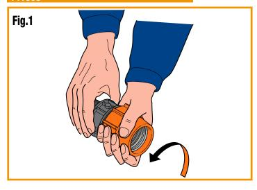
Shown here as fully assembled. Loosen the <u>retaining nut</u> and the <u>circular conduit retainer.</u>
