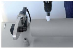
Check that the welder and die pairs have reached the correct operating temperature of 500°F (260°C).
