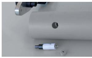
Insert the male die pair into the pipe hole until the concave part touches the outer surface of the pipe.
