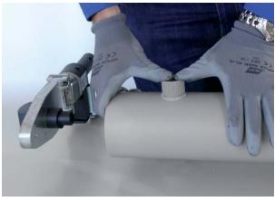
After a cooling time of 10 minutes, the new joint can be pressure tested or placed into operation.
