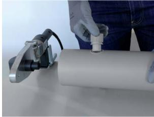
Once the heating time is over, immediately insert the welding saddle into the heated hole without turning. The fitting must be perfectly fixed and pressed against the pipe surface for about 30 seconds.
