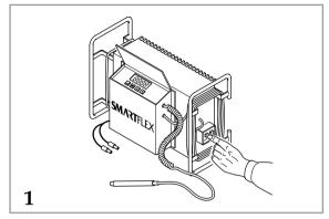
CONNECT THE WELDING UNIT LEADS TO THE FITTING. (FITTING AND PIPES MUST BE PREVIOUSLY INSERTED IN THE ALIGNER)
