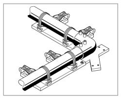
ASSEMBLE PIPE BUTTS AND SOCKET AND LOCK IN PLACE WITH THE ALIGNER
