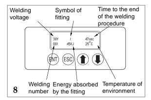
WHEN THE WELDING CYCLE BEGINS, WELDING DATA APPEAR ON THE DISPLAY
