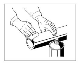
DEGREASE PIPE AND FITTING WITH PAPER WIPES SOAKED IN PRIMER LIQUID
