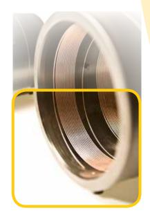
Electrofusion is the thermal junction process between pipe and fitting obtained by heating a resistance wire included in the fitting. The fittings have a resistive wire inside which is connected to the outside cable terminals.
