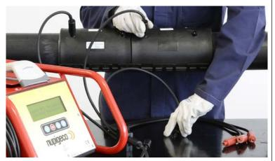
10 Connect the other cable of the electrofusion machine to the connector slot of the <u>red triple cable</u>.
