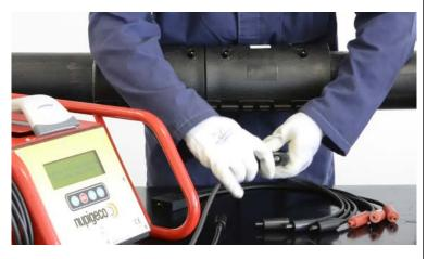
Connect 2 connectors of the <u>black triple cable</u> to the first pin marked "A" of each module. The third connector doesn't need to be used.
