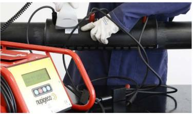
13 After the welding cycle is positively completed, mark the actual time on the modules and disconnect all the cables.
