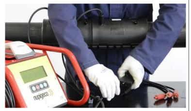
**11** Connect 2 connectors of the <u>red triple cable</u> to the second pin marked "B" of each module. The third connector doesn't need to be used.
