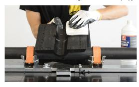
**6.** Install the two half shells on the pipe, keeping the bead in the center.
