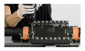
**9.** In any case before starting the fusion process, fit the alignment clamp and check if it is firmly secured on either side of the 'BFRS'.
