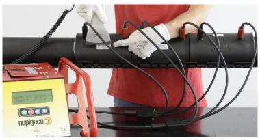
16 After the welding cycle is positively completed, mark the actual time on the modules and disconnect all the cables.
