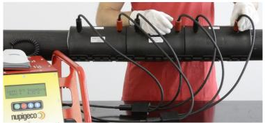
15 Perform welding: scan with the optical pen the barcode on EIVLRS I module and proceed with welding.
