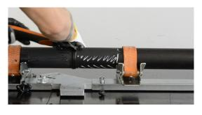
**4.** Clean the pipe surface with isopropyl alcohol (minimum concentration 91%).
