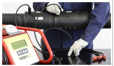
10 Connect the other cable of the electrofusion machine to the connector slot of the red triple cable.
