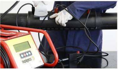
13 After the welding cycle is positively completed, mark the actual time on the modules and disconnect all the cables.
