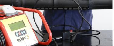
12 Perform welding: scan with the optical pen the barcode on EIVLRS I module and proceed with welding.
