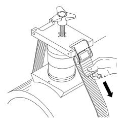
**4.** Insert the belt up in the buttonhole and then pull down to tighten the 'top load' saddle on the pipe.
