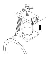
**2.** Insert the positioning tool into the "top load" saddle and place them on the pipe, after completing scraping and cleaning operations (check installation instruction of the fitting).
