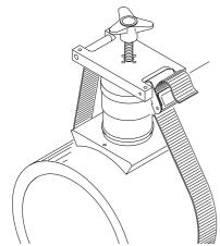
**3.** Pass the belt under the pipe and insert it into the tightening clamp from the bottom to the top, as showed on the figure.
