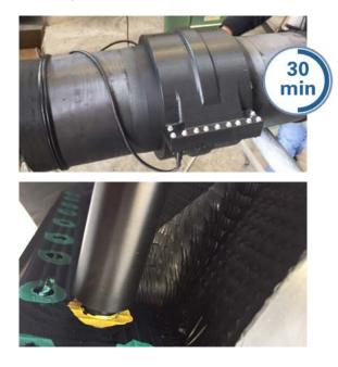
**11.** Connect the welding unit with the other two pins of the lateral zones. Scan the barcode of the lateral zones and start the welding.
