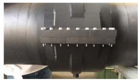
**9.** In any case before starting the fusion process, fit the alignment clamp and check if it is firmly secured on either side of the BFRS.
