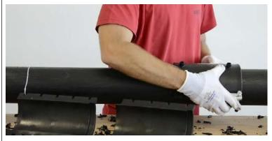
Place the first underclamp on the very end of the assembly: hook the square holes of the underclamp to the teeth on the side of the module; align the two screws to the corresponding holes, line up the metal spacer and use a wrench to tighten the two screws until they are in position **A** in the lower part (feel the screws sticking out of the bottom - see figure in the circles below). Repeat the operation with the second underclamp in the consecutive position.
