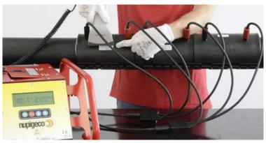
After the welding cycle is positively completed, mark the actual time on the modules and disconnect all the cables.
