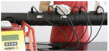
Perform welding: scan with the optical pen the barcode on EIVLRS I module and proceed with welding.
