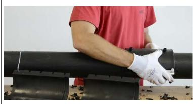
Place the first underclamp on the very end of the assembly: hook the square holes of the underclamp to the teeth on the side of the module; align the two screws to the corresponding holes, line up the metal spacer and use a wrench to tighten the two screws until they are in position A in the lower part (feel the screws sticking out of the bottom - see figure in the circles below). Repeat the operation with the second underclamp in the con-
