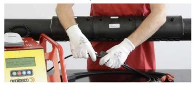
12 Connect each connector of the <u>black triple cable</u> to the first pin marked "A" of each module.
