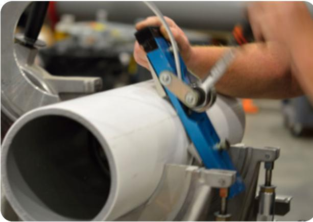
**NIRON Clima Cool-pro** is a pipe produced using PPR material with an outer layer of **POLYPROPYLENE duly UV stabilized** with a dedicated masterbatch.
