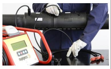
10 Connect the other cable of the electrofusion machine to the connector slot of the red triple cable.
