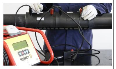
12 Perform welding: scan with the optical pen the barcode on EIVLRS  ${
