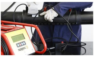
After the welding cycle is positively completed, mark the actual time on the modules and disconnect all the cables.
