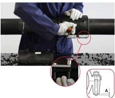
$\overline{7}$  Place the terminal module <code>EIVLRS</code>  ${ t T}$  on the scraped pipe, adjacent to the previous one just installed: the lip at the end of the module must overlap the protruding edge of the previous one. Install the first underclamp across the two adjacent modules (follow the instruction on Step 6). Then install the second and third underclamps in the consecutive positions (follow the instruction on Step 6). The terminal module EIVLRS T\_must always be the final
